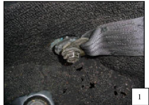
2. Position the hole toward the rear of the car, with the fat end toward the inside of the car (driver's side shown). Insert the anchor end of the seatbelt upward through the slot in the seatbelt adapter (see photo).
