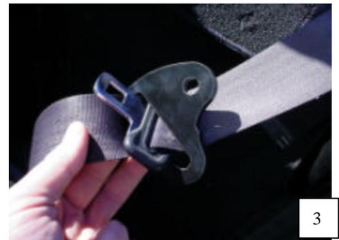
4. Unbolt the stock seatbelt guide from the rollbar tab using a 9/16" wrench.
