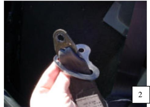
3. Slide the adapter up to the male end of the buckle and manipulate the buckle through the adapter's slot. This may require some effort, but the buckle must be able to fit through the slot. If it doesn't fit through, DO NOT proceed further\*.
