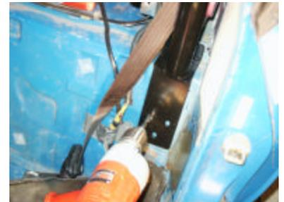
18) **Drill the rear mounting foot holes and install the backer plates.**
