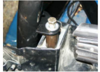
17) **Drill the front foot support holes and install backer plates.**
