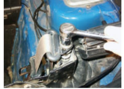
9) **Remove the ECU (if installed) and cut off top stud.**
